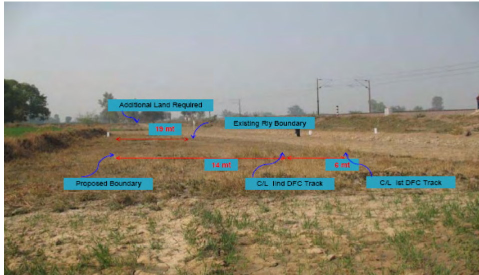
Fig - 2.4 Typical layout of land having DFC and existing Railway track
